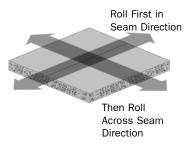
Continue this process until floor is complete. When seams are complete, use a 75 lb. carpet roller to roll entire floor starting with the seam (or seams.) Roll first in seam direction and then across seam direction.
